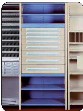
Modular drawer installation should have a shelf directly above and below the drawer guide support as shown.
